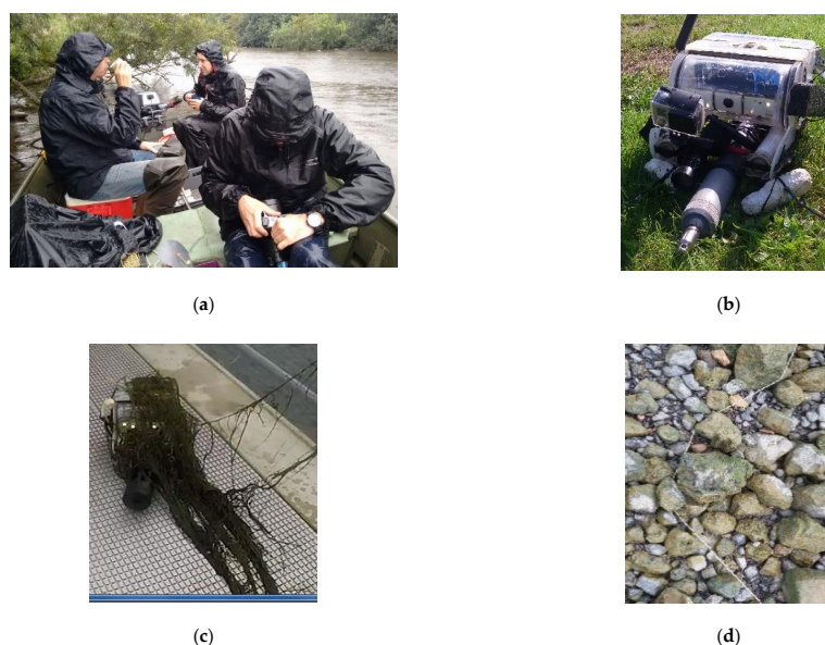
Figure 4. Field challenges: (a) operation under rain conditions, where a laptop is needed to operate some drones, (b) adjusting the buoyancy of small drones with heavy sensors is a time-consuming task; (c) excess of vegetation blocks thrusters; (d) tether tangled in rocks/obstacles.
