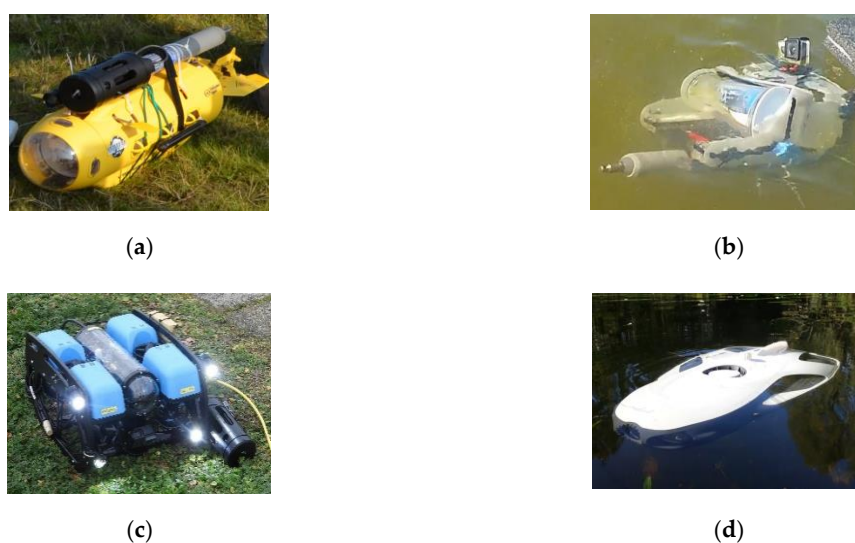
Figure 1. Illustration of multiple underwater drones equipped with cameras, lights, or water quality sensors. (a) Neptune; (b) OpenROV 2.7; (c) BlueROV2; (d) PowerRay.
