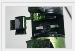
FluoroProbe III with Hydro-Wiper after weeks of operation
